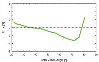
Mean **cosine response** of four Apogee SE photometric sensors. Cosine response was calculated as the relative difference of SE photometric sensors from the mean of replicate reference photometric sensors deployed outdoors. These data are the average of the AM and PM response.
