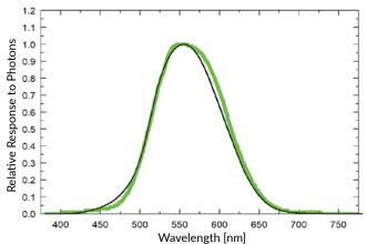
Spectral sensitivity of photometric sensors. Replicate (n=6) sensors indicate a spectral shift to lower wavelengths caused by non-zero incidence angle, resulting in mismatch between CIE 1931 photopic weighting factors and sensor sensitivity. Measurements were made with CR6 datalogger at 10 nm increments in the monochromator.
